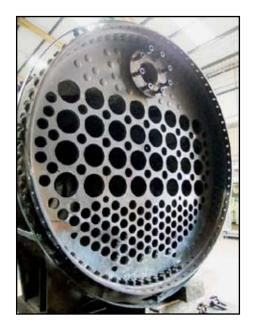
Sir Keith Park's boiler requires 112 Small Tubes, and the Superheater 32 Flues in which are placed 32 Elements, which will cost around £38,000. Here's your chance to sponsor an item which will see the loco return to service in 2011.
